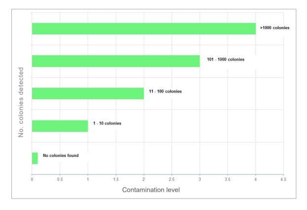
Following graphs show the contamination levels found in the polluted fuel samples after treatment with FPB-77. The "kill rate test" was performed at determined intervals and conclusions drawn assess the number of active colonies in various samples. In all the samples, the biocidal action of Hydra FPB-77 was effective for at least 26 weeks.
